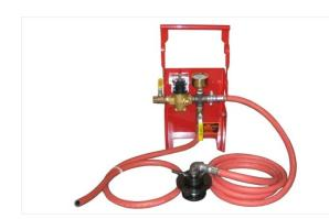
T51750 Cooling System Test Kit for GE and EMD Engines This kit is designed to introduce 20 PSI water pressure to the cooling system via the water tank fill neck. The fill neck pressure fixture is placed on the fill neck the same as the locomotive pressure cap and a spring is then compressed to ensure a positive seal at 20 PSI. Other pressures can be utilized depending on railway mechanical specifications from 0-25 PSI.
